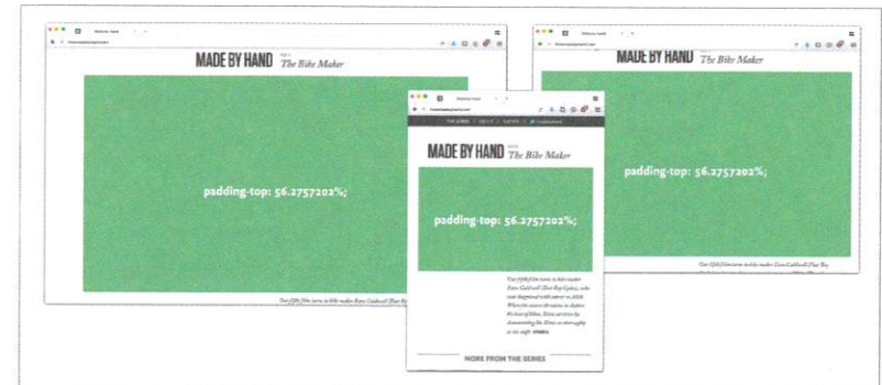
FIG 3.8: As we resize our padding-top -enabled box, it maintains the shape and proportion our video needs, without a single scrap of content inside.
