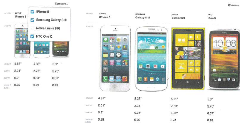
FIG 1.8: An example of the jQuery mobile Column Toggle table pattern, with the same table shown at narrow and wide widths.
