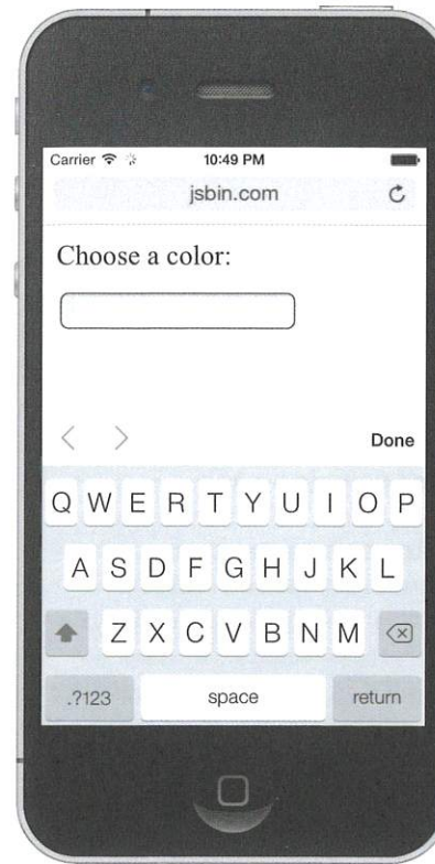
FIG 1.18: A color input falls back to a plain text input in iOS 7.
